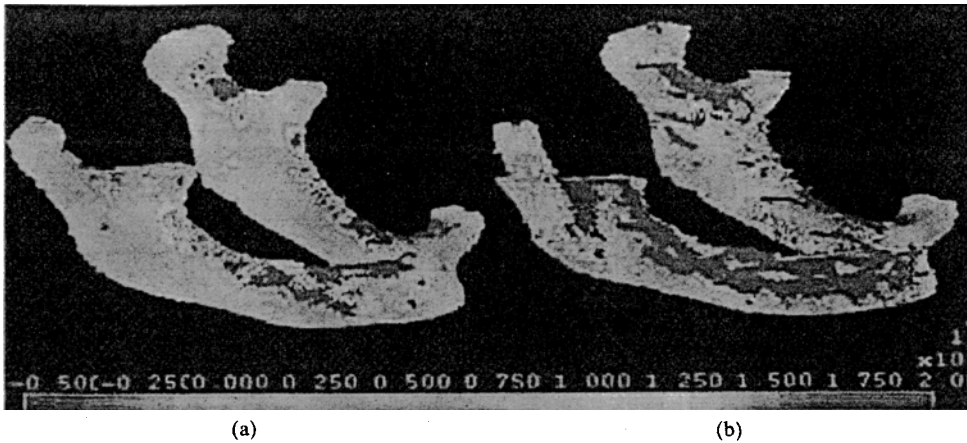
Fig. 5 Maximum principal stresses for the normal mandible (a) and the CCRG mandible (b). The superior border of the mandible experiences high tensile stresses in both cases due to the bending deformation. However, stresses in the CCRG mandible are significantly higher than the normal mandible. The condyle experiences very low tensile stresses in the normal mandible. The rib graft experiences moderate tensile stresses (up to 8 MPa) in the CCRG mandible. Note horizontal scale numbers should be multiplied by 10
